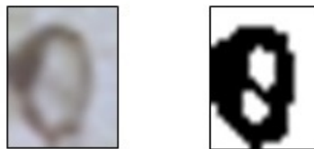
Figure 4.1.: Air bubble sample image (left) and binary thresholded image (right), Threshold value (T) = mean pixel value
