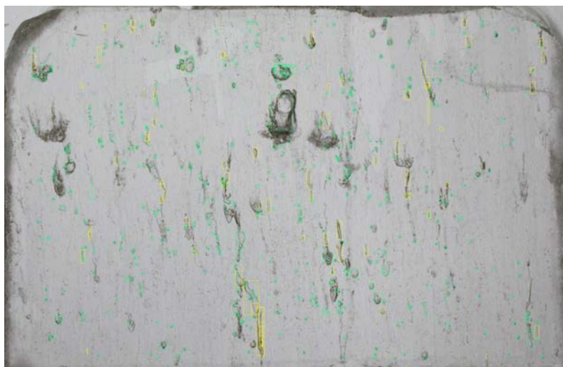
Figure 3.19.: 5th section from top of multiyear ice core 1 obtained from N-ICE2015 Campaign (A.4) after air bubble and channel detection; width:10cm; height:6cm
