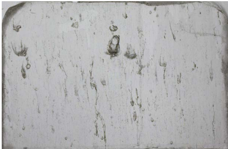
Figure 3.18.: 5th section from top of multiyear ice core 1 obtained from N-ICE2015 Campaign (A.4) before air bubble and channel detection; width:10cm; height:6cm
