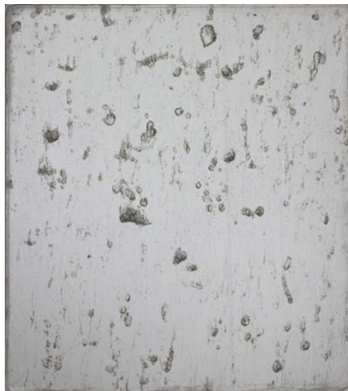
Figure 3.16.: 4th section from top of multiyear ice core 1 obtained from N-ICE2015 Campaign (A.4) before air bubble and channel detection; width:10cm; height:11cm
