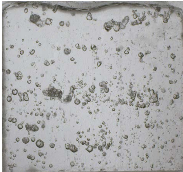
Figure 3.12.: 2nd section from top of multiyear ice core 1 obtained from N-ICE 2015 Campaign (A.4) before air bubble and channel detection; width:10cm; height:9cm
