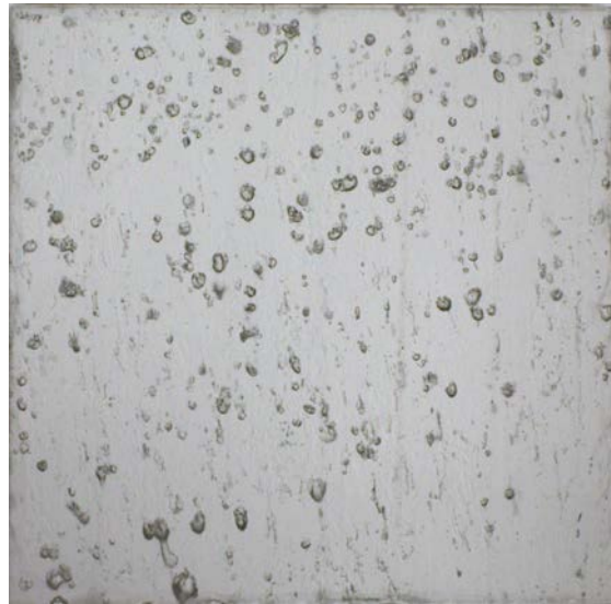
Figure 3.14.: 3rd section from top of multiyear ice core 1 obtained from N-ICE2015 Campaign (A.4) before air bubble and channel detection; width:10cm; height:9cm
