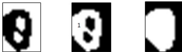
Figure 4.3.: Binary thresholded image (left), binary inverted image (middle)(detected contour marked by 1), cavity filled image (right)
